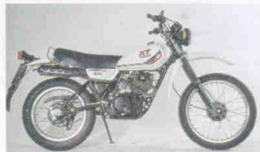
XT 250 (1980-1990): Zweiventil, 17 PS, Kickstarter. Cantilever-Schwinge, Trommelbremsen, 8-l-Tank, 124 kg.
